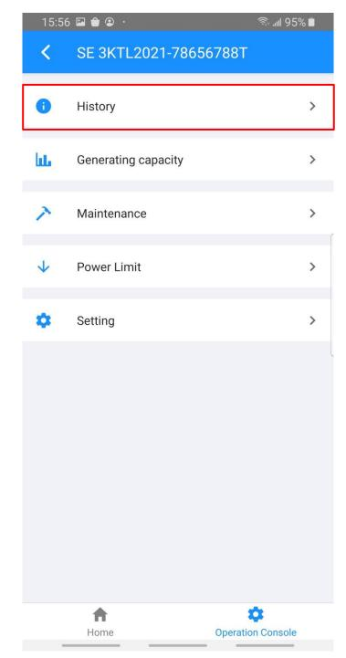
Press **Operation Console** at first and then Press **History** to go to the history log page ( as shown below ). It contains all the logs for the inverter.
