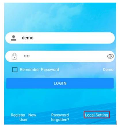
Press **Local Setting** to go to the connect page. This page shows the inverters which you can connect or you have connected. ( As shown below )
